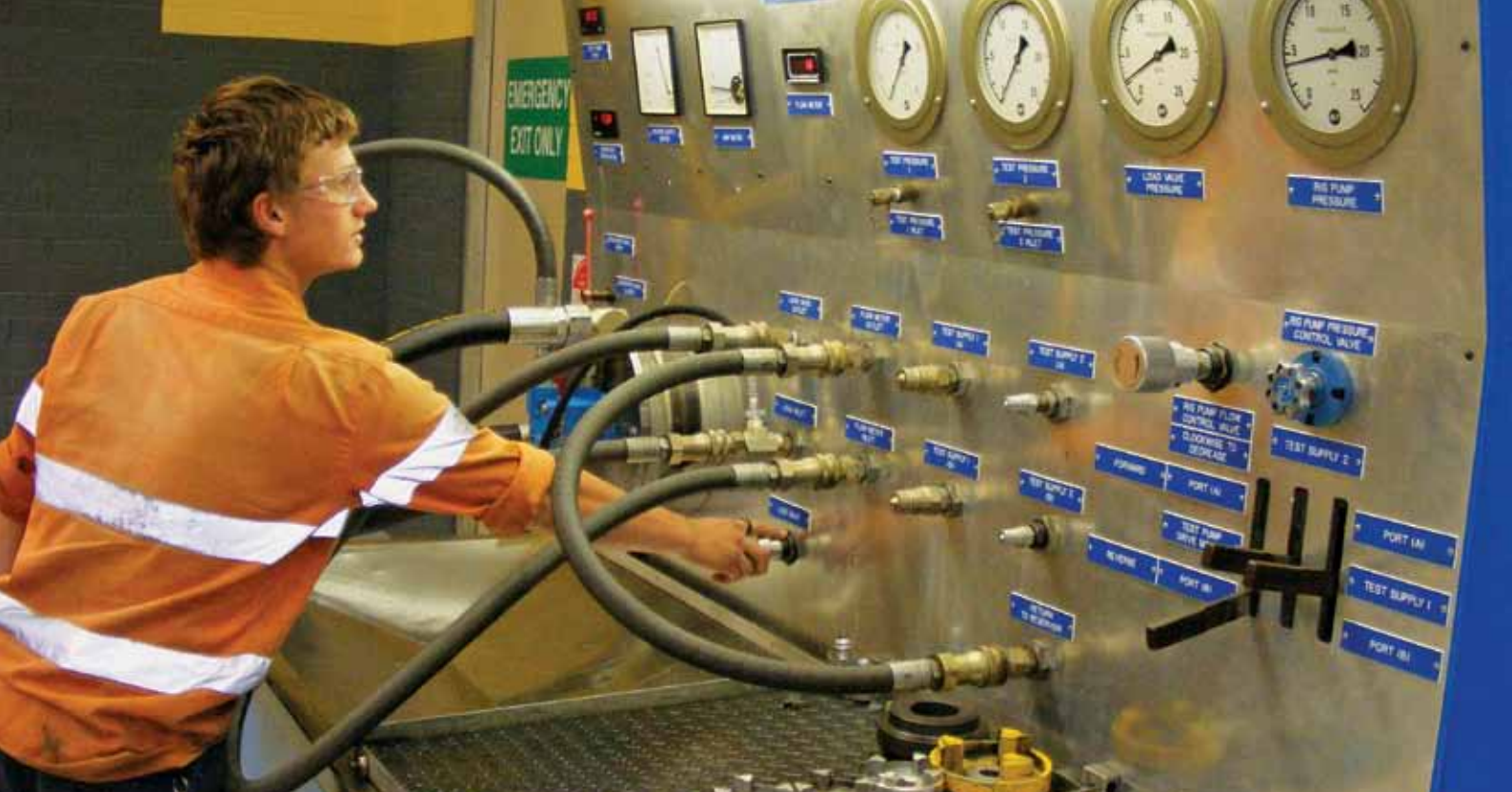
On completion of pump repair, students test the pump efficiency rate. Here a student puts the pump through its paces. Photo: Polytechnic West.
