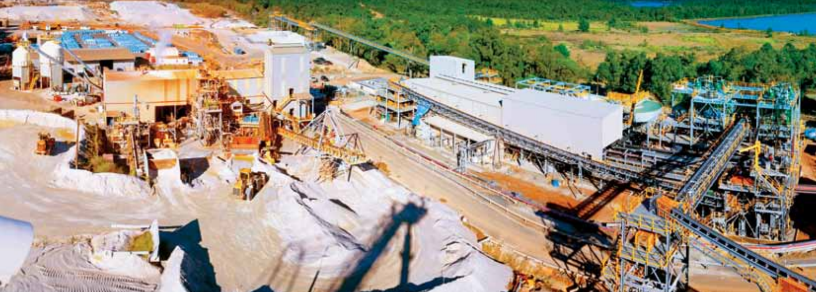
The original crusher (left) which now processes the higher-grade lithium, and the new crusher (right).
