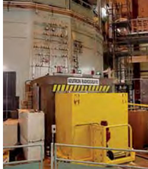
The neutron radiography facility at the Nuclear Energy Corporation of South Africa experimental reactor
