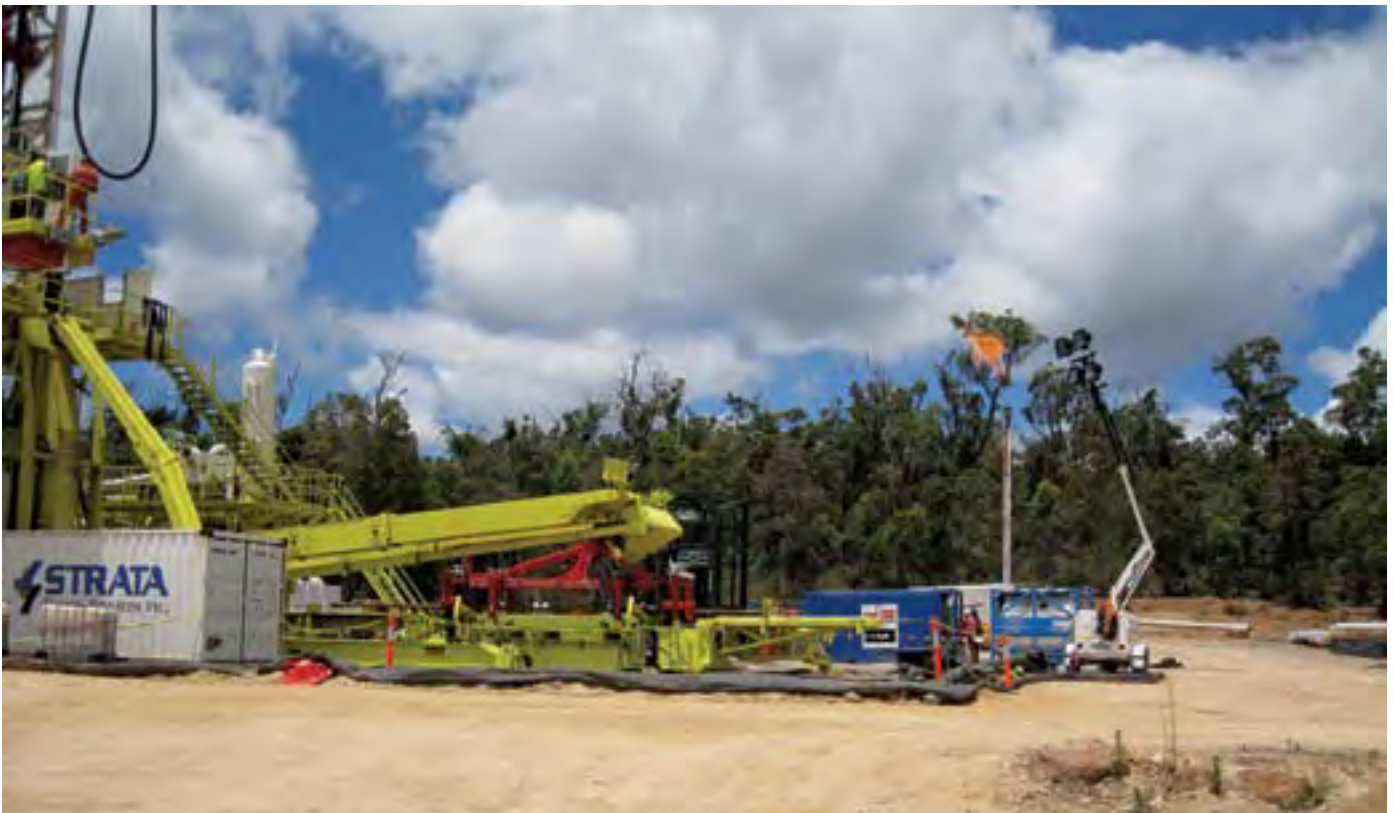
Flaring gas while conducting pressure managed drilling at Whicher Range 4
