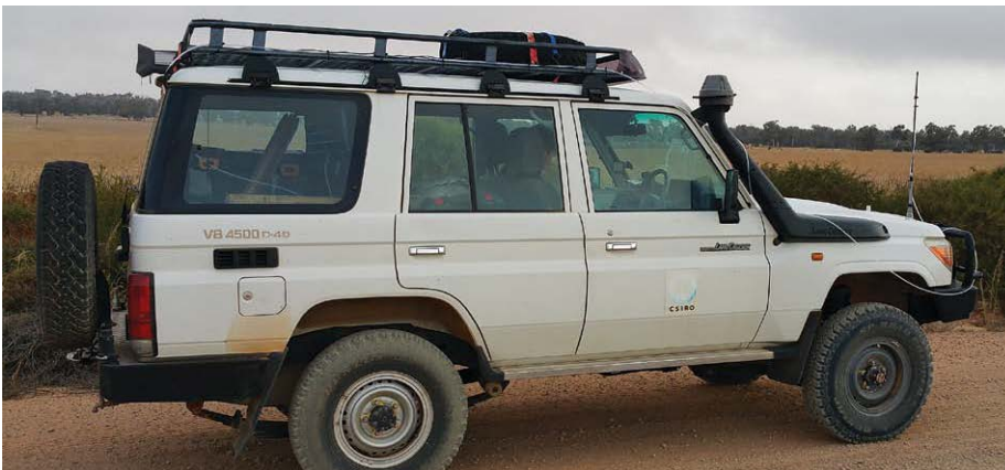
CSIRO 4WD with the mobile methane sensing equipment.
