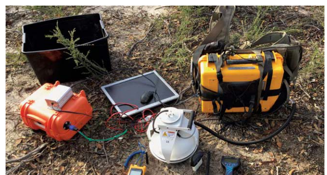
Soil methane flux measuring equipment used by the CSIRO.
