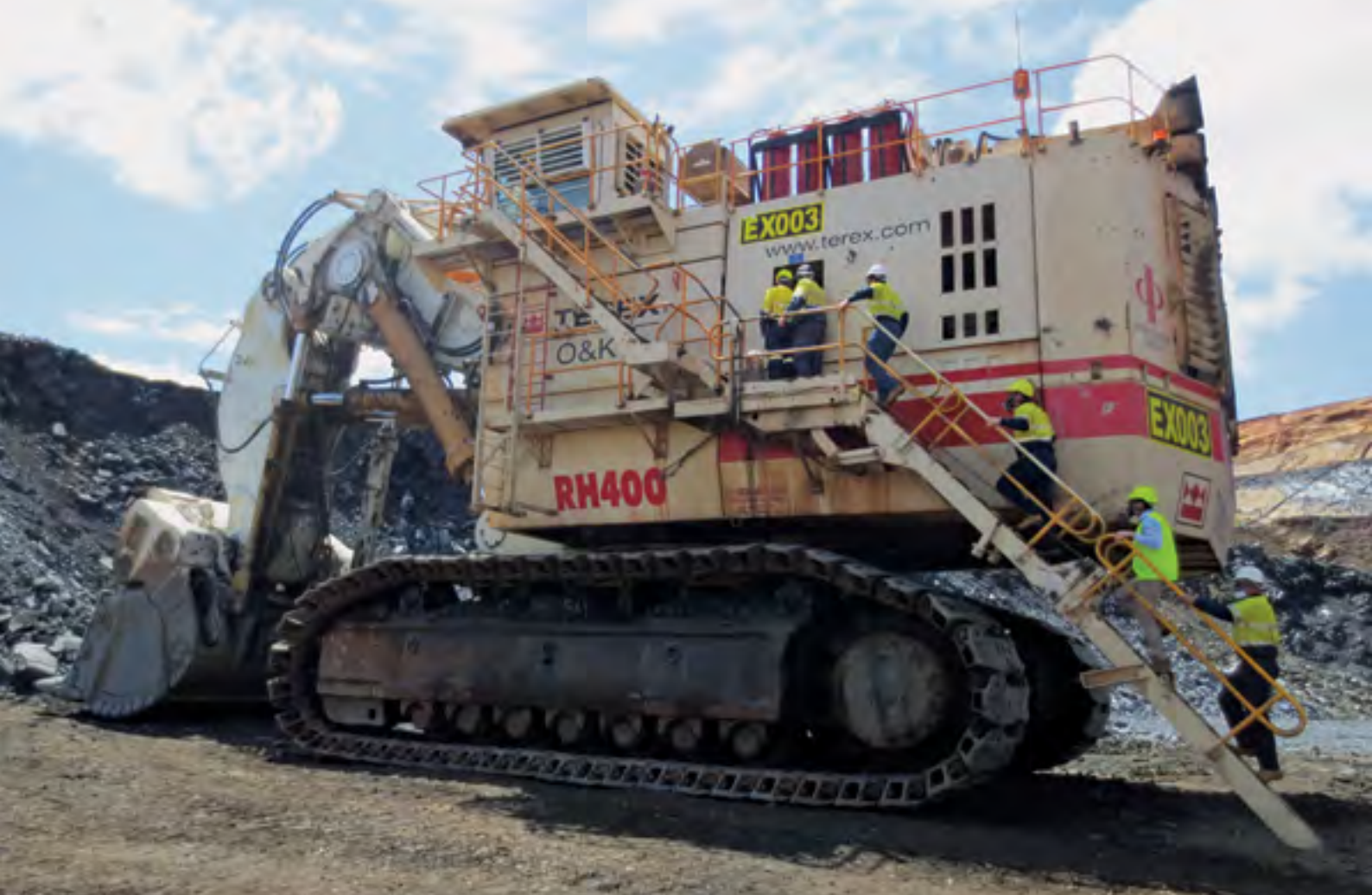
The 980-tonne Terex RH400 hydraulic excavator.
