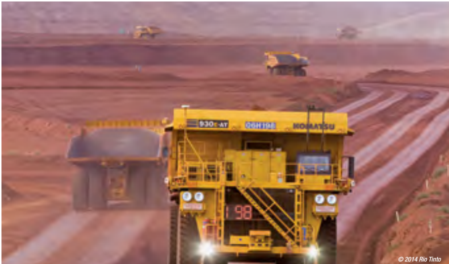
Autonomous haul trucks in operation at Rio Tinto's West Angelas mine site.
