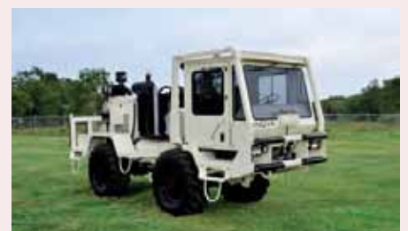
One of the National Geosequestration Laboratory’s Curtin University-based vibroseis trucks used for seismic survey research.
