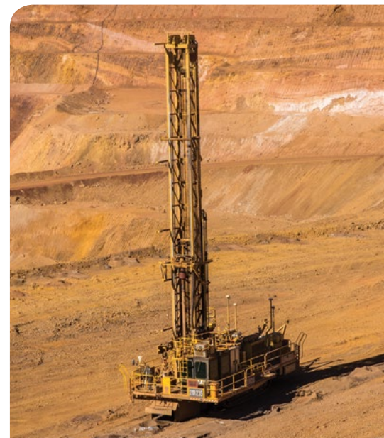
Autonomous drilling at Rio Tinto's West Angelas mine in the Pilbara. Photo: Rio Tinto
